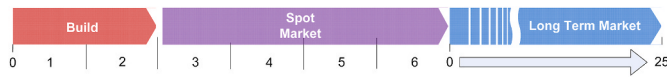
Fig. 5. Base Case scenario: Immediate construction of the power plant with a duration of two years followed by four years of short term spot market sales at PLD prices.
